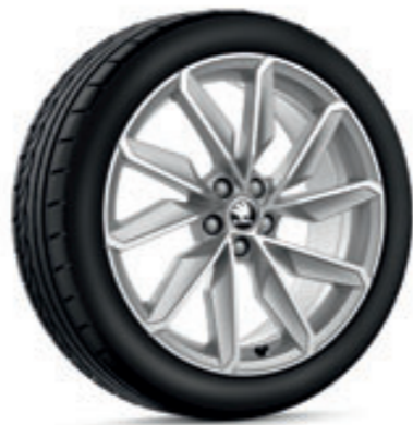
Blade light-alloy wheel silver metallic, brushed 7.0J x 18" ET39 for 205/45 R18 654 071 498AE 8Z8 654 071 498D 8Z8*
