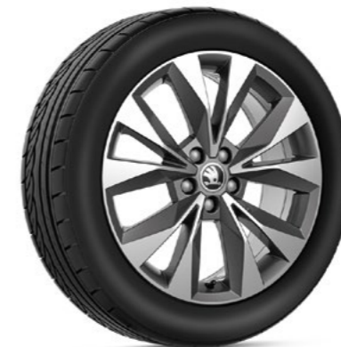
Geneva light-alloy wheel anthracite metallic, brushed 6.5J x 17" ET40 for 205/50 R17 654 071 497G HA7 654 071 497AE HA7*
