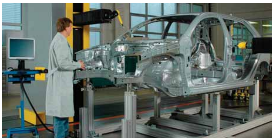
Measuring vehicle body part dimensions on digital measuring device
