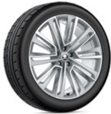
AQUARIUS front alloy wheel 8.5J × 21" ET40 for 235/45 tyre rear alloy wheel 8.5J × 21" ET40 for 235/45 tyre* 5LG 071 491 8Z8 | silver metallic brushed rear alloy wheel 9J × 21" ET42 for 255/40 tyre** 5LG 071 491A 8Z8 | silver metallic brushed
