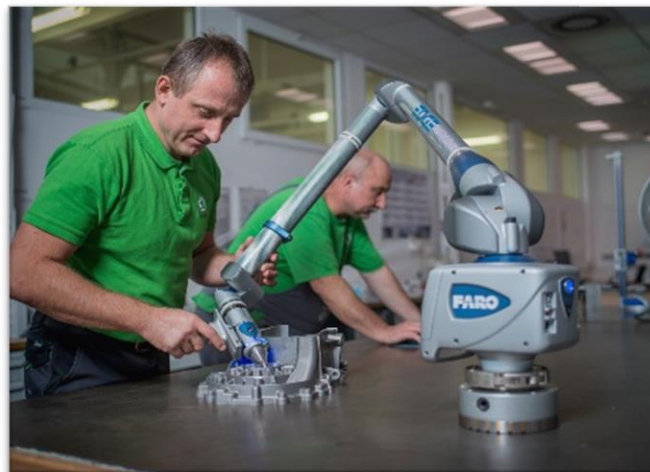
Measuring with 7-axis FaroArm
