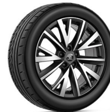
Gigaro light-alloy wheel black metallic, brushed 7.5J × 18" ET40 for 235/55 R18 57H 071 498A FL8 57H 071 498F FL8*
