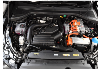
Orange-coloured cables in the engine compartment
